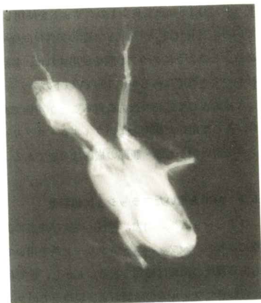
Fig. 16 A flying parakeet (body length = 8 cm) using a soft flash X-ray with a V_c of 80 kV, an A-C distance of 3 mm, and an F-F distance of 1.4 m.
