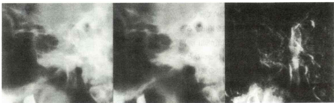
Fig.5 Comparison among Frame #1 (left), the background estimated by LIP (center), and the subtraction result (right). The subtracted gray levels are magnified by three for display.
