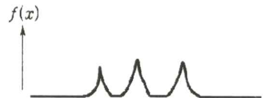
Fig.2 Configuration after top-hat transform.
