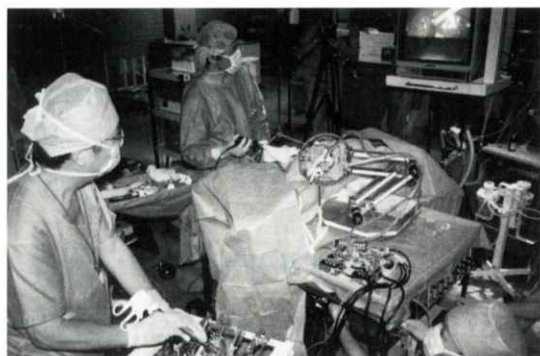
Fig.4 In vivo test of remote minimally invasive surgery system
