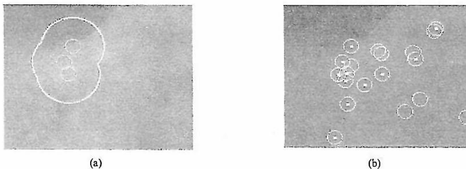
Figure 10: Comparison of the performance between VRF and ANN. A mass contained no microcalcifications was misdetected as a cluster with three FP microcalcifications (a). The missed FP detections can be eliminated by ANN (b).
