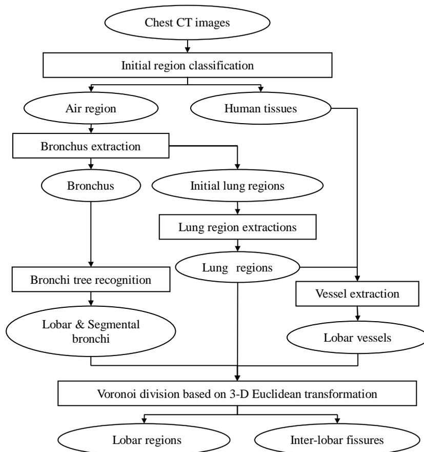
Fig. 1. Processing flow of lung lobe and fissure extractions.
