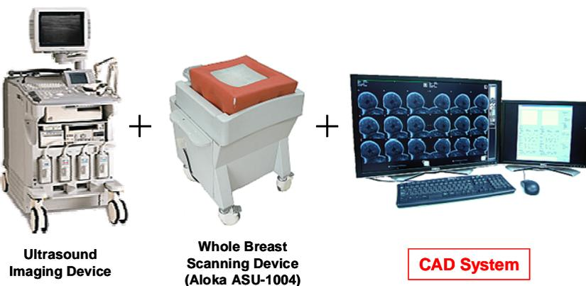
**Fig. 10.** An overall system for breast cancer screening using ultrasound images. The system consists of an ultrasound imaging device and a whole breast scanning device for whole breast volumetric data acquisition. A workstation is also included for the purpose of pre-processing and analysis of the images acquired by the scanning device from the patient and as a viewer for the visualization of the images along with the CAD results [16].
