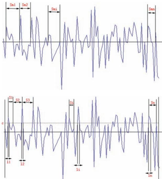
Fig. 3. Feature definition of  $S_m$ ,  $S$  and  $T_p$ .
