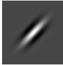
Fig. 2. Gabor filter function ( \sigma = 4.30 , \gamma = 0.45 , \lambda = 13.0 )
